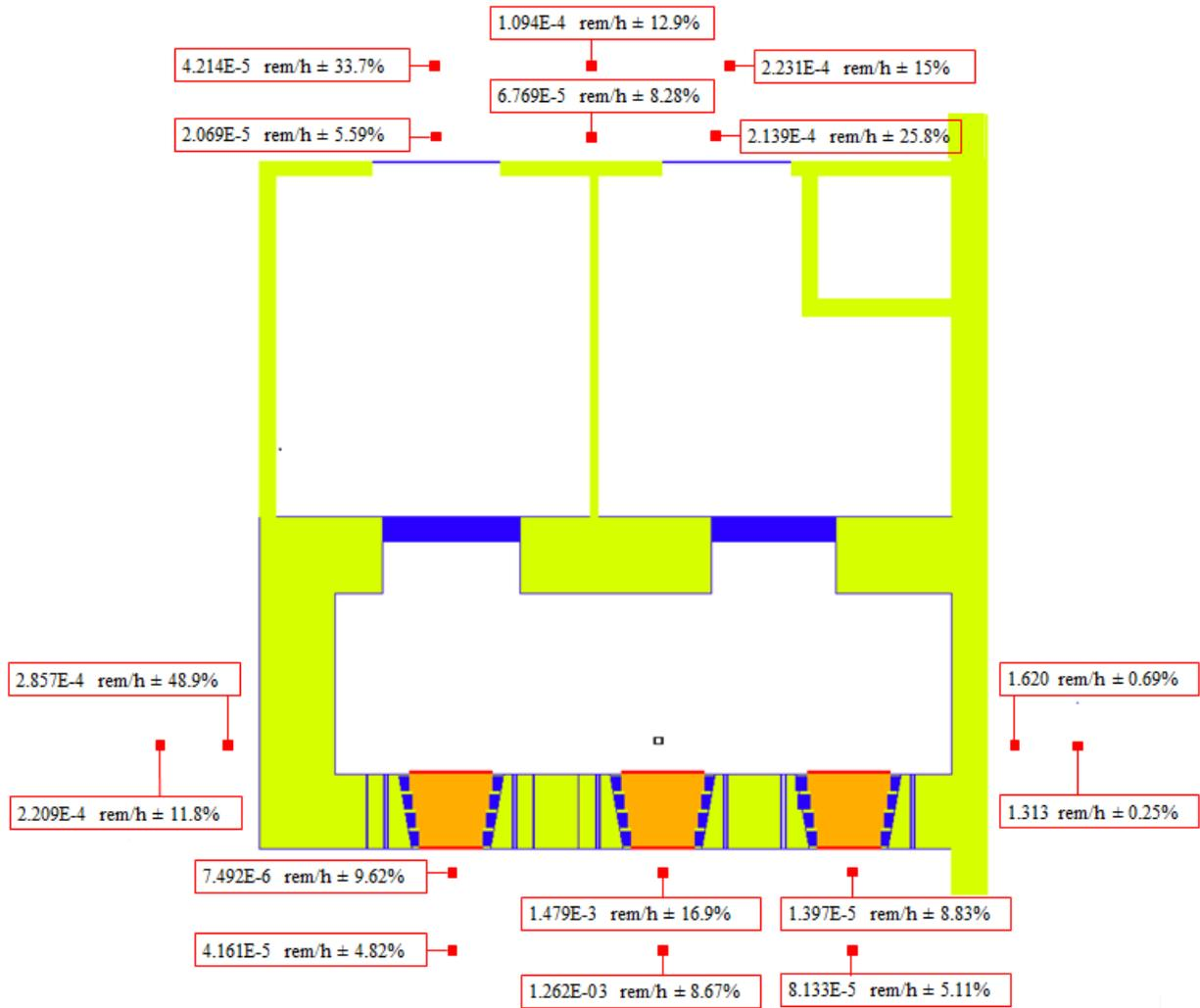
Fig. 7: Dose rates immediately after the bombardment with normal concrete for the right wall.
